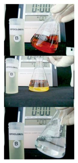
Figure 2 - Changing of the solution color from orange to colorless
