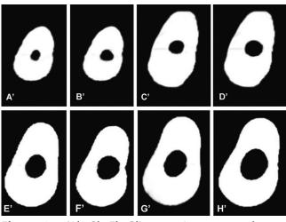
**Figure 1** – (A', C', E', G') are uninstrumented cross sectional images and (B', D', F', H') are instrumented cross sectional images at 4 mm, 6 mm, 9 mm, and 12 mm respectively prepared with hand ProTaper files
